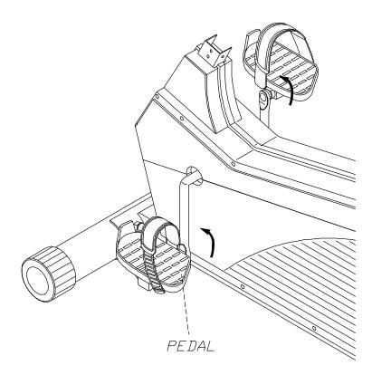
**5.** Attach pedals (35, 36). Axles of pedals are branded "L" and "R." The pedal marked "R" goes on the right hand side of the bike and the one marked "L" on the left hand side. Tighten the left pedal by turning counter-clockwise and the right pedal by turning clockwise.
